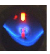
the flame. The temperature rise of the flame is directly translated into a reading expressed as a percentage of the lower explosive limit (% LEL/LFL). This measuring principle is unique in its uniform re-
